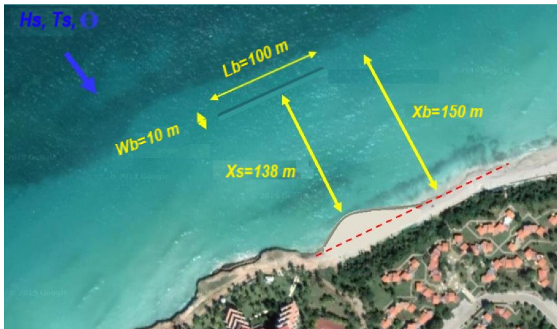
Figure 28. Formation on the beach of a 12 m wide spit due to the location of a 100 m long submerged breakwater. Source: Author's own.
