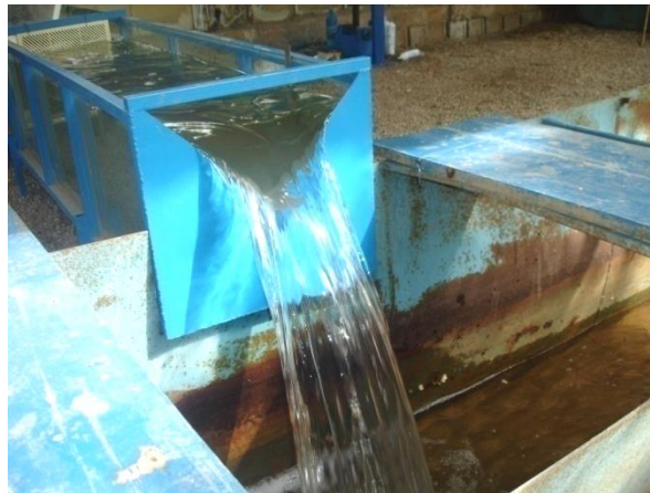
Figure 2. Measurement of the flow discharged from the vortex tube with a 90° weir.
