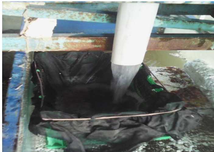
Figure 5. Flow discharge tube, diversion sediment and collection of sediment.
