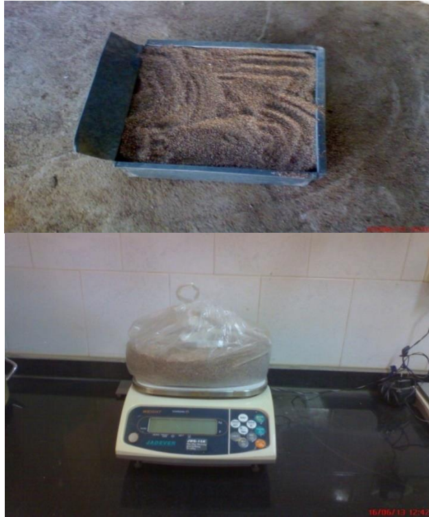
Figure 4. Laboratory process for obtaining the granulometric curve.
