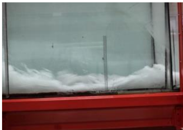
Figure 8. Beginning of hydraulic jump in 70 l/s.
