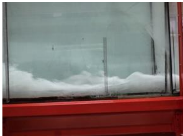
Figure 7. Beginning of hydraulic jump in 90lit/s.
