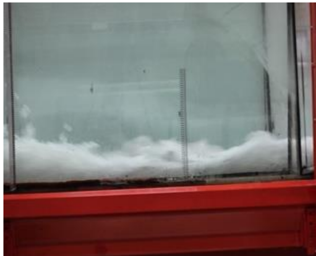
Figure 9. Beginning of hydraulic jump in 50 l/s.
