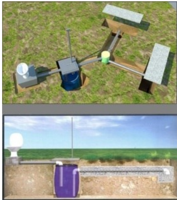
Figure 1. General scheme (plant and profile) of the Popular Ecological Toilet (ENSOME – PIENSA UNI, 2012).
