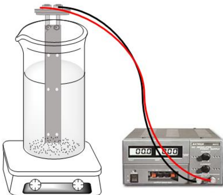
Figure 1. Electrochemical cell used for the electro-oxidation process
