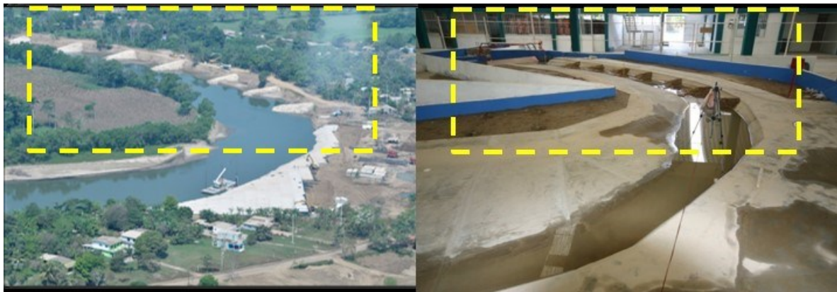
Figure 2. Prototype and physical model of the Sabanillas diversion channel, located in the Municipality of Centro, Villahermosa, Tabasco, México.
