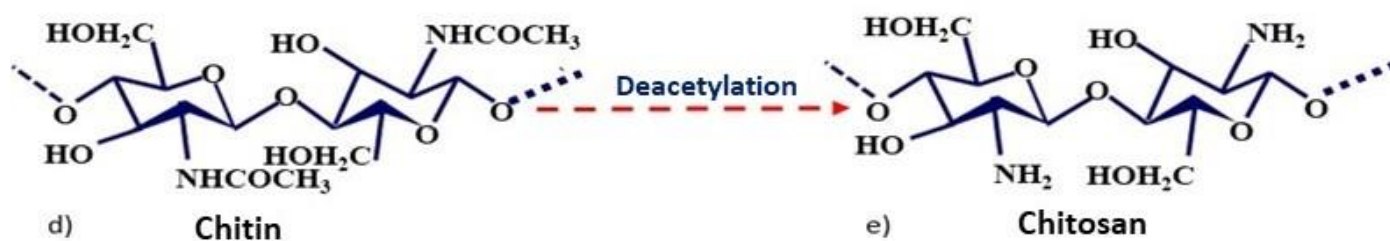
Figure 1. Molecular structure of alginate a) basic units of \alpha -L-guluronic acid (G), \beta -D-manuronic acid (M); b) blocks of the essential acids; c) alternating sequences of the MG blocks; d) Molecular structure of chitosan chitin, and (e) chitosan.
