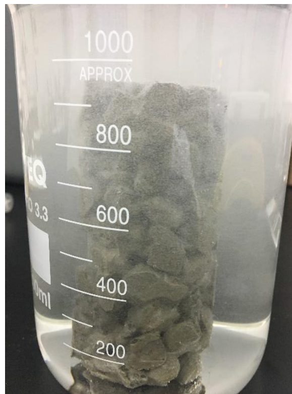
Figure 3. Deposition of heavy metal precipitates in concrete in a batch reactor.
