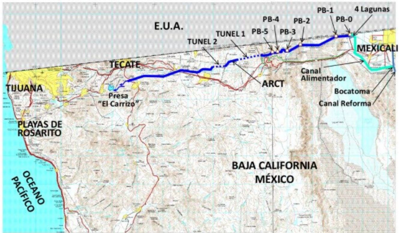
Figure 1. Location of Tijuana and the Colorado River-Tijuana Aqueduct (ARCT). PB-0 to PB-5 are pumping plants 0 to 5. Source: Comisión Estatal del Agua de Baja California (2011).
