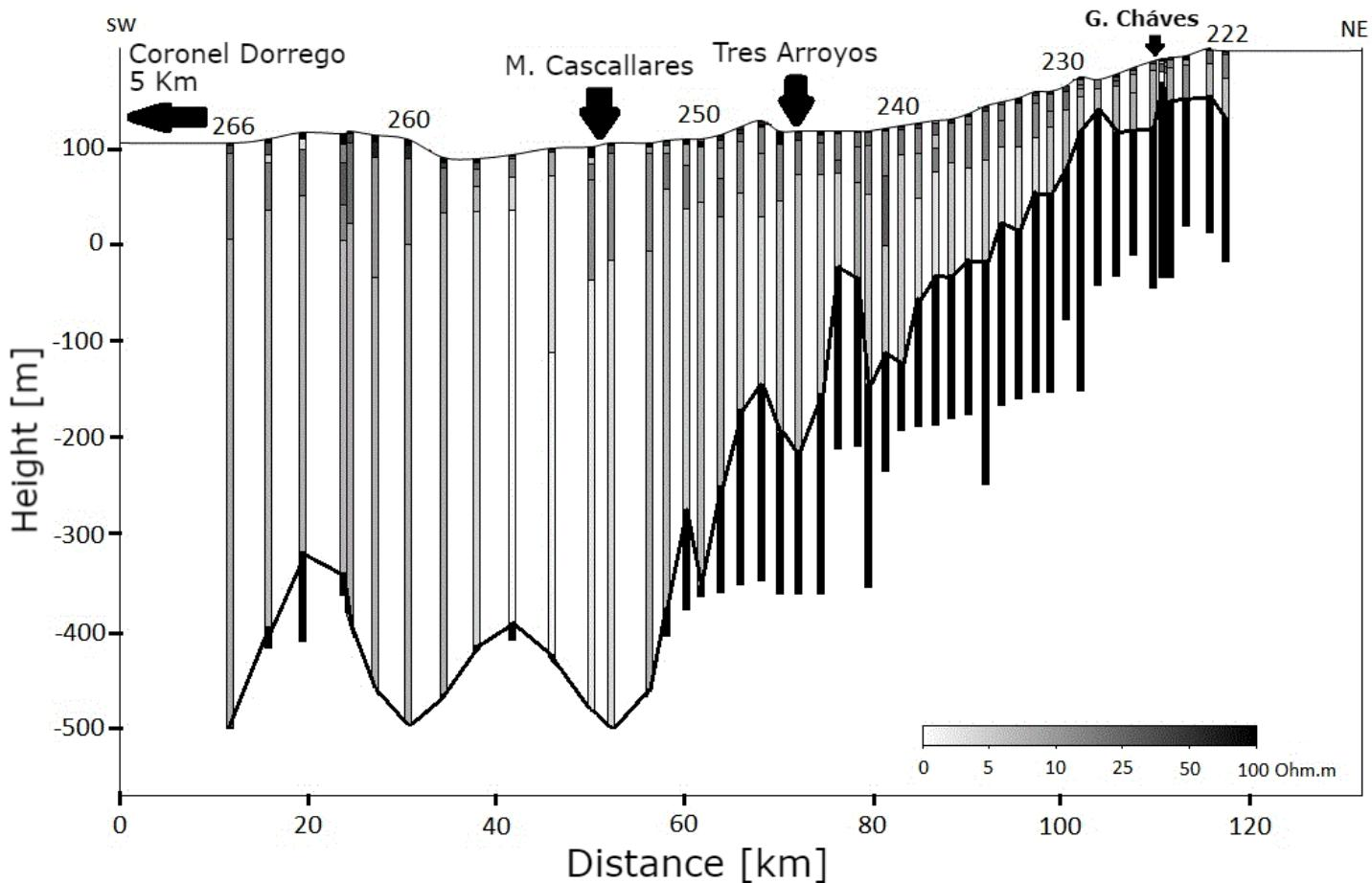
**Figure 4.** Results of the 49 inverted VES with their regional references, resistivity, and depth. The black curve represents the modeled depth for the resistive basement.
