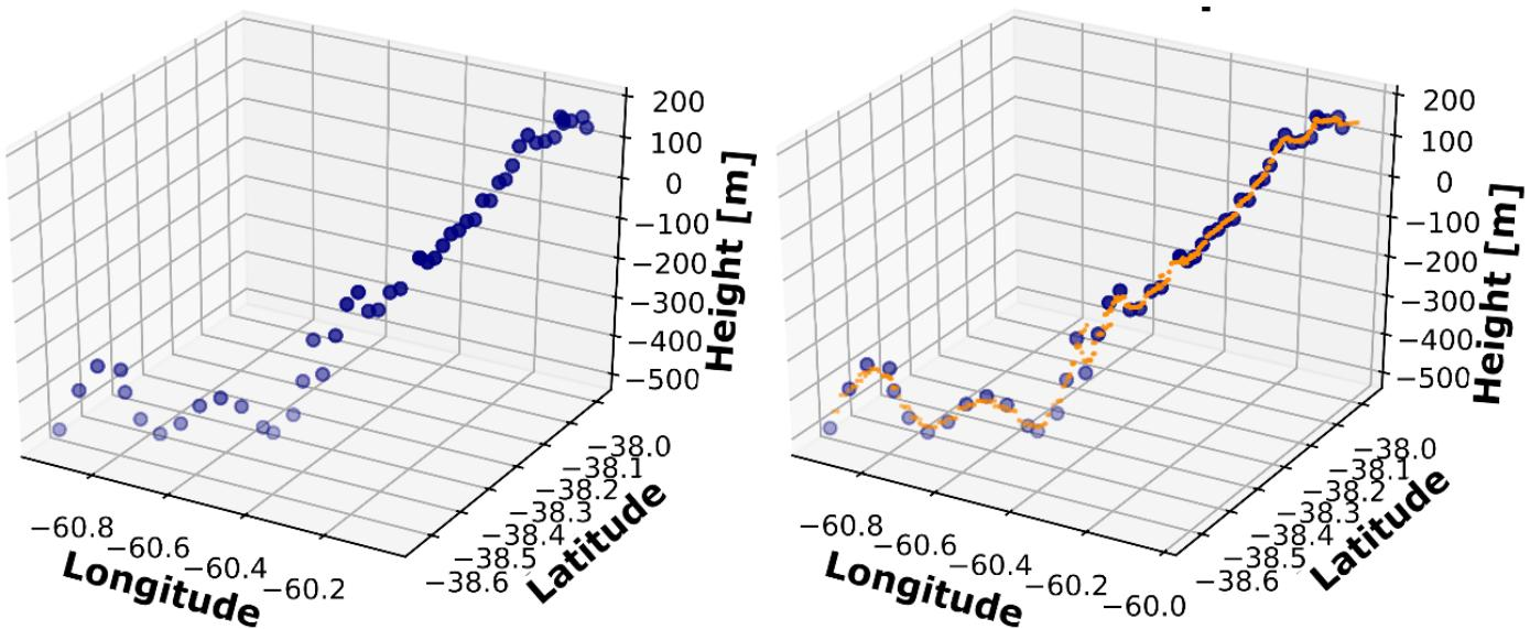
**Figure 5.** Three-dimensional representation of the true basement depths obtained by VES. The image on the left shows in blue the heights taken from the reference ellipsoid. The image on the right adds in orange the
