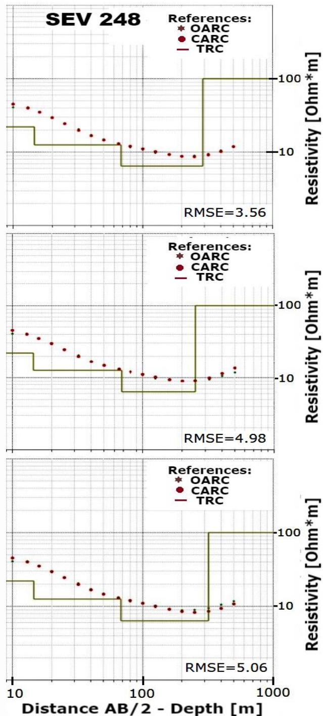
**Figure 6.** The VES 248 has its OBD at 270 meters, with an RMSE = 3.6 % (upper figure). By reducing the true depth of the basement, to 250 meters we reach the proposed tolerance (center figure), similarly at 320 meters if
