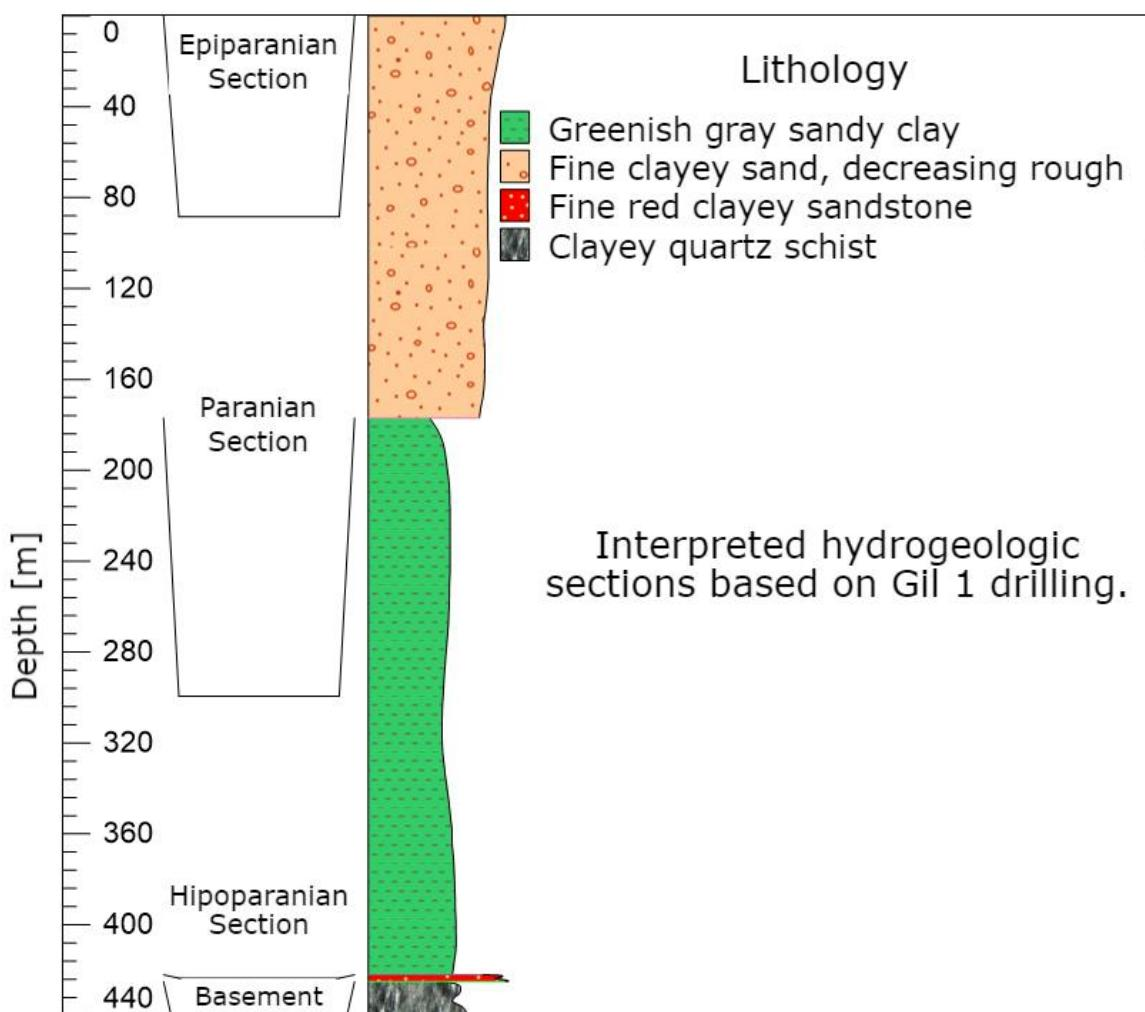
**Figure 2.** Interpretation of hydrogeological sections based on well drilling Gil 1 (Dirección Nacional de Geología y Minería, 1970). The basement is only reached less than a meter deep in the bottom hole, here it is shown extended.
