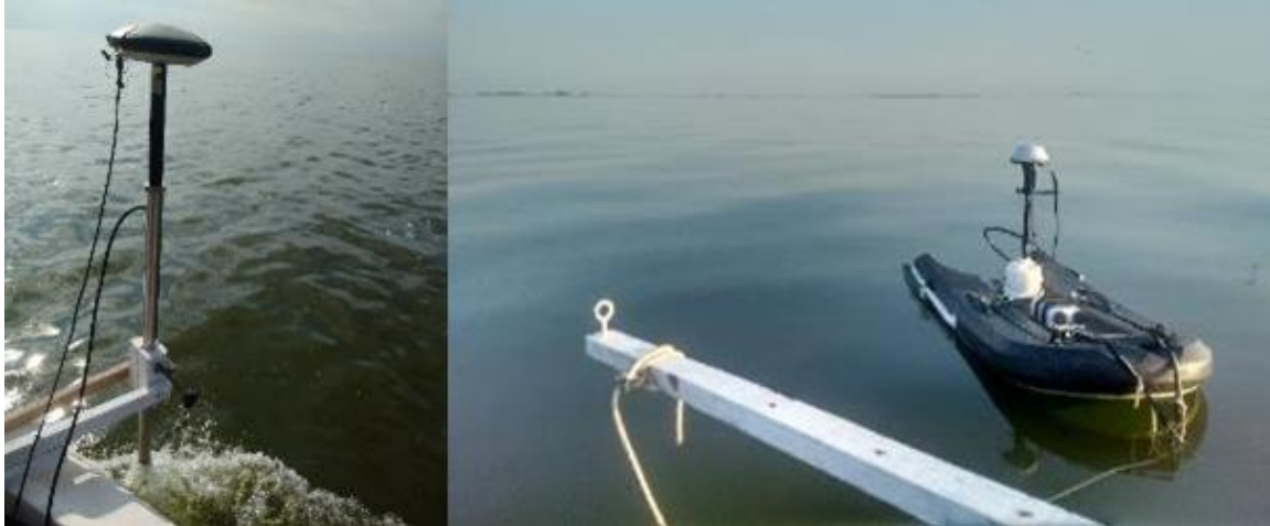
Figure 3. Instruments. Left: GPS equipment and submerged echosounder; right: ADCP Sontek M9.
