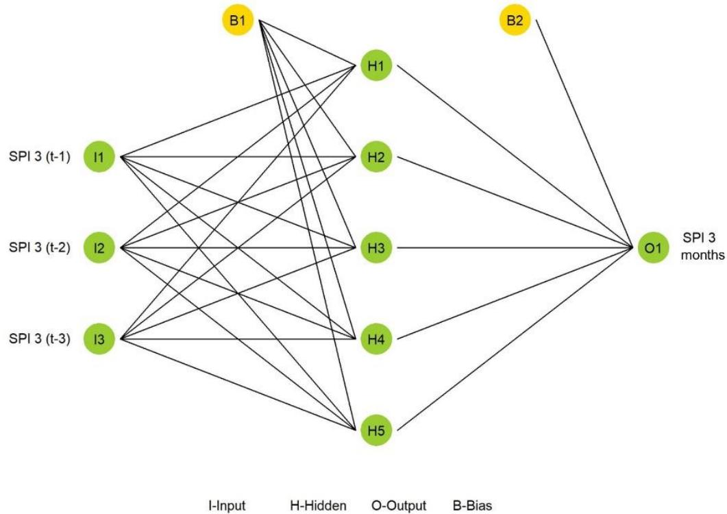
**Figure 4.** The architecture of the neural network for SPI 3 of group 2a.
