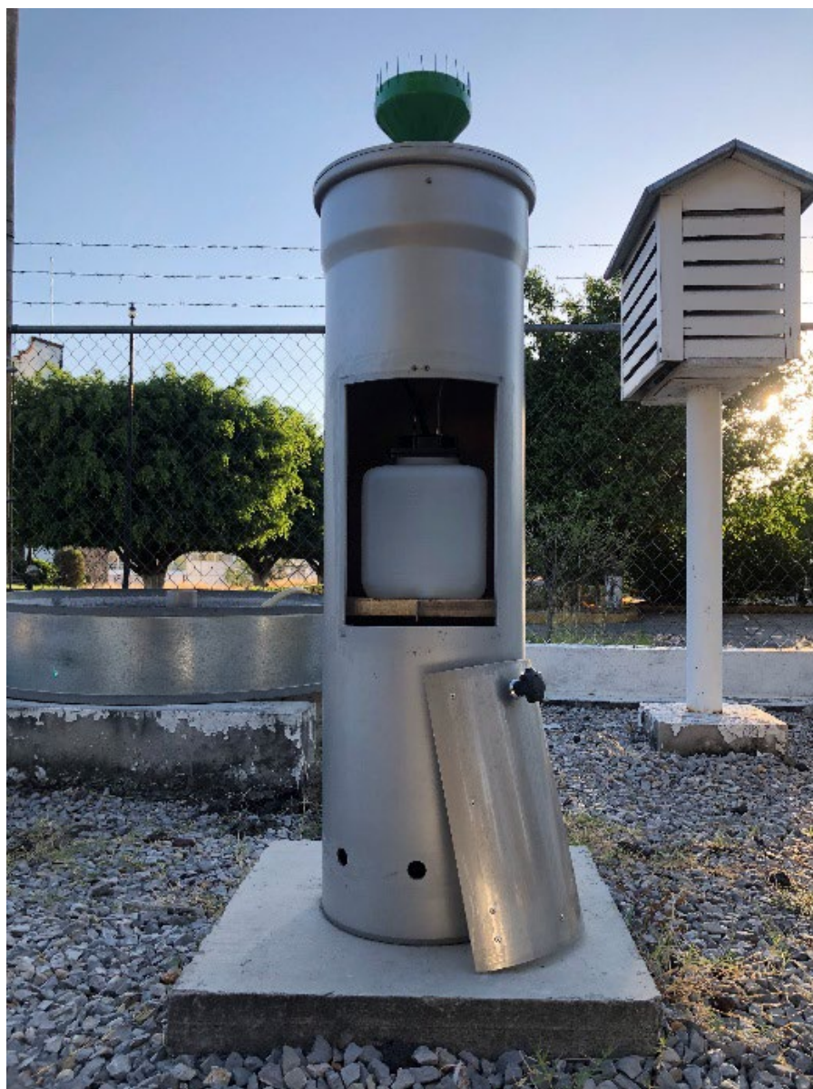
Figure 4. Rainwater collector RS2 PALMEX.
