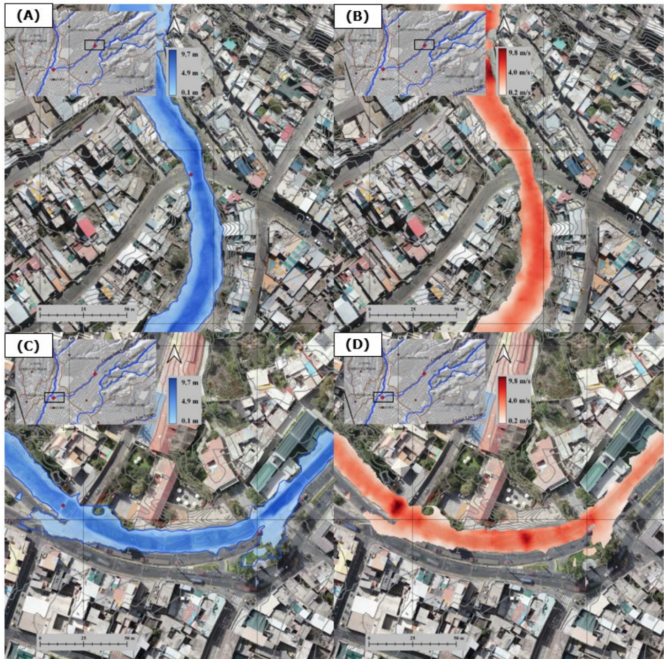
Figure 19. Flood hazard map, for a return period of 100 years A), B) water depth and speeds on the Cahuide bridge; C), D) water depth and velocities in Av. Juan de la Torre of the San Lázaro gully, using the HEC-RAS numerical model.
