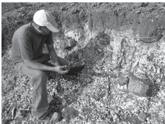
Figure 15. Appearance of leachates in a gully downstream from San Jose de Avino.
