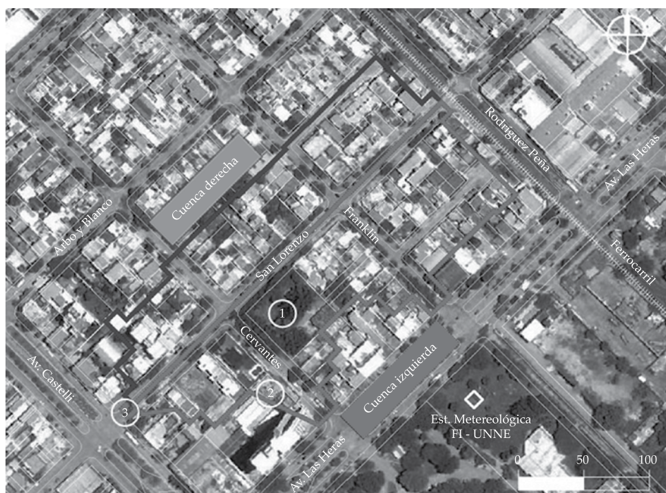
Figure 3. Micro-watershed containing sinks in San Lorenzo Street and Castelli Avenue. References: 1) exposed soil, 2) construction tower, 3) sampling sites (upstream from the drain entrances).
