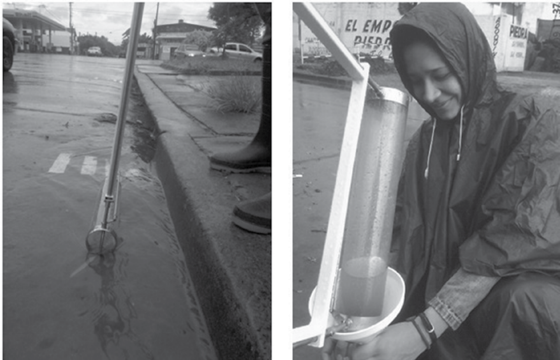
Figure 10. Collection of samples with a DHL collector.
