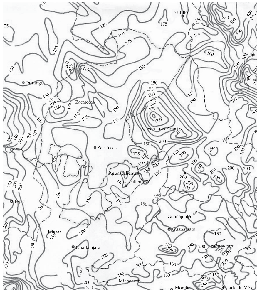
Figure 6. Maximum isocontour lines for a return period of 1000 years, state of Zacatecas (SRH, 1976).
