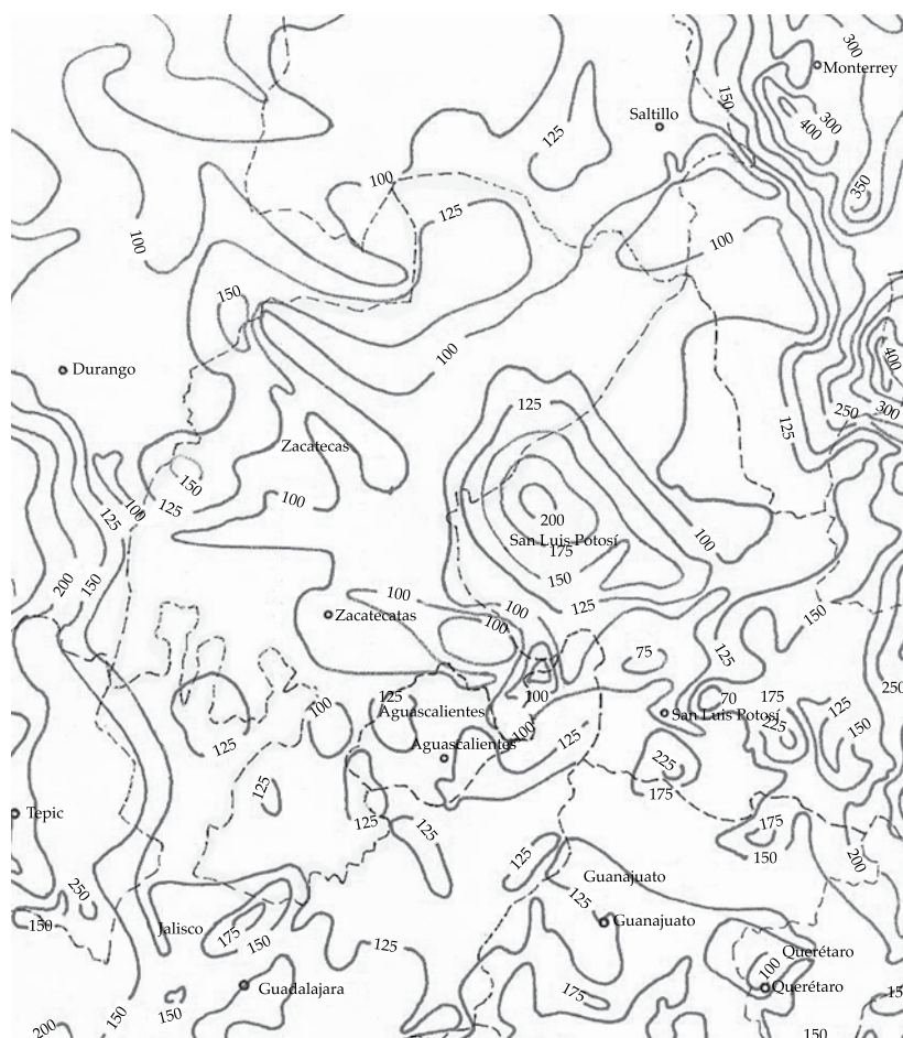
Figure 5. Maximum isocontour lines for a return period of 100 years, state of Zacatecas (SRH, 1976).
