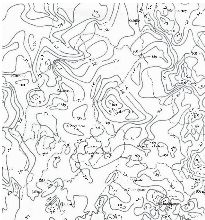
Figure 7. Maximum isocontour lines for a return period of 10 000 years, state of Zacatecas (SRH, 1976).
