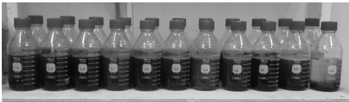
Figura 1. Preparation and mounting of batch reactors in the laboratory.
