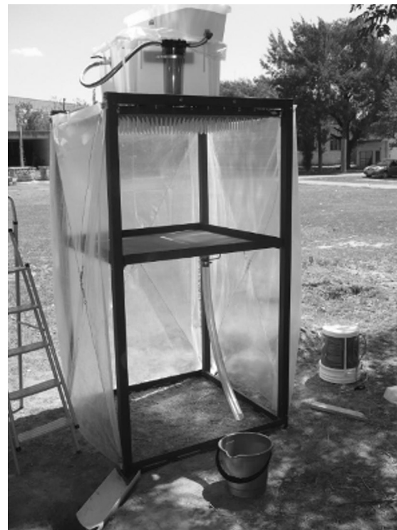
Figure 1. Rainfall simulator in the field.
