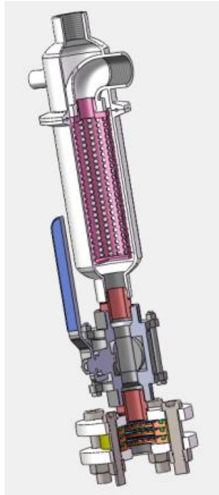
**Figure 3.** The cross-section diagram of the filter module.
