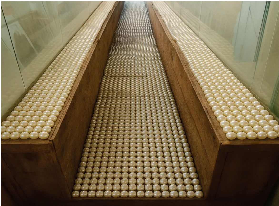
Figure 2. Compound cross-section in the experimental channel with roughened main and minor beds using uniformly arranged plastic spheres for studying hydraulic jump characteristics.
